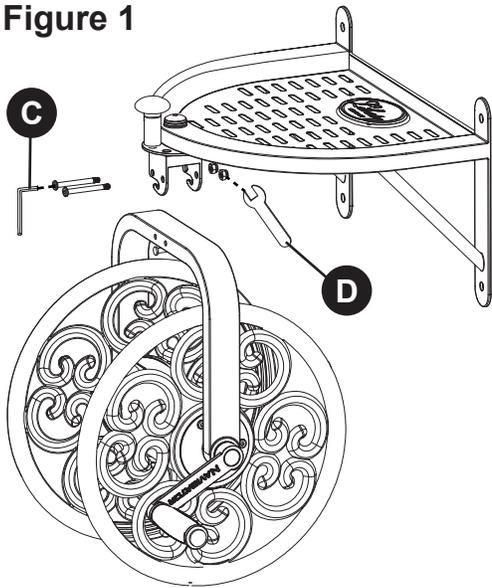
1. First, remove Spool from Yoke by using supplied 4 mm Allen Wrench (C) to hold Allen Bolts in place while using supplied Wrench (D) to remove Lock Nuts. Remove Allen Bolts from holes. To remove Spool from Yoke, lift the Spool upward, then guide it out of small slot on Yoke. Set Spool on ground. **See Figure 1.**
